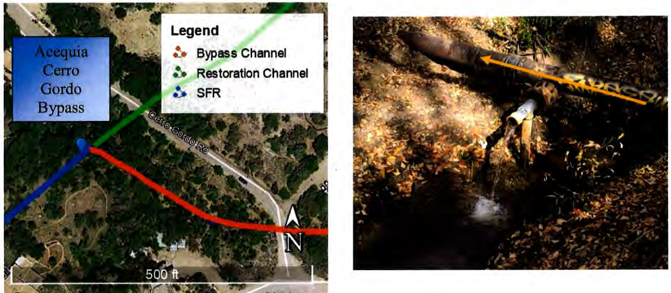
Figure 18. Location map of Acequia Cerro Gordo Bypass (left); Cerro Gordo Bypass 3-in. outlet pipe (open), looking upstream* (right)
