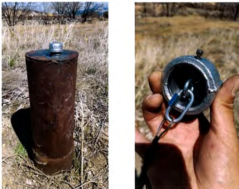
Figure 46. USGS observation well at Frenchy’s Field (left) and pin-locked cap where transducer cable is attached (right)
