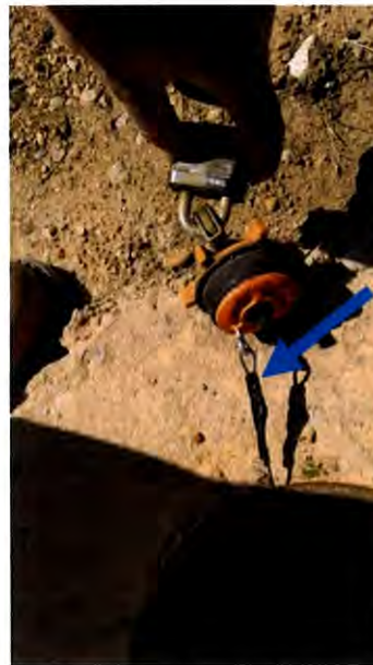
Figure 42. SFRMW-02 monitoring well (left), and well plug with arrow indicating where transducer cable is attached (right), 3/22/19
