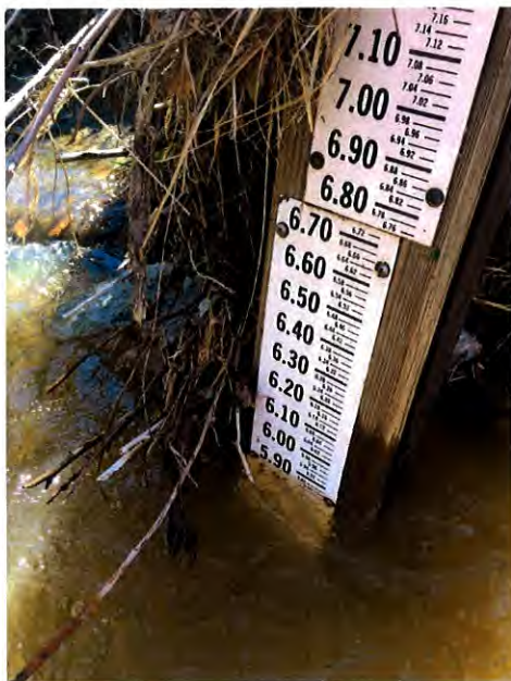
Figure 29. Staff gage just upstream of stilling well (left) and SFR looking upstream at St. Francis Gaging Station (right)
